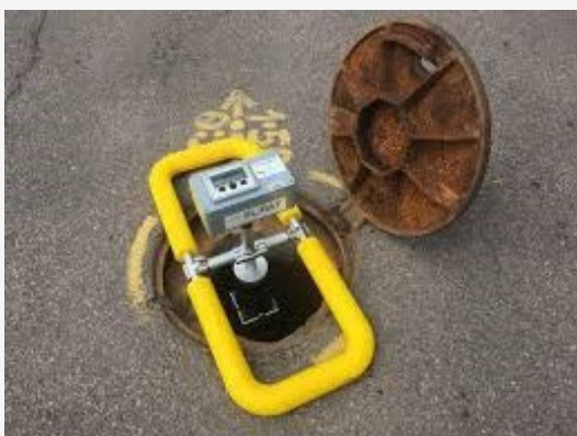
SL-RAT transmitter unit at manhole
