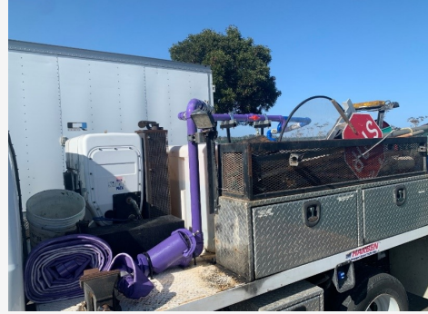
Harben water truck with purple piping for recycled water and blue pipes for potable water
