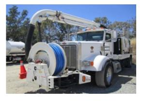
Fortunately, this incident occurred at night when sewer flows are low. Taking advantage of this timing, Noel and Phil were able to contain the flow utilizing the District's Vac-Con vehicle. The Vac-Con is a "combination" specialized sewer vehicle that can vacuum, jet and store wastewater in its 1,500-gallon tank.
