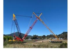
The crane assembly also includes extra truss pieces that are installed as needed to extend its reach (photo left).
