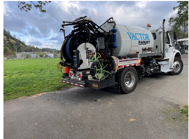
The Vector Ramjet is used by the Maintenance Crew to clean pipes
