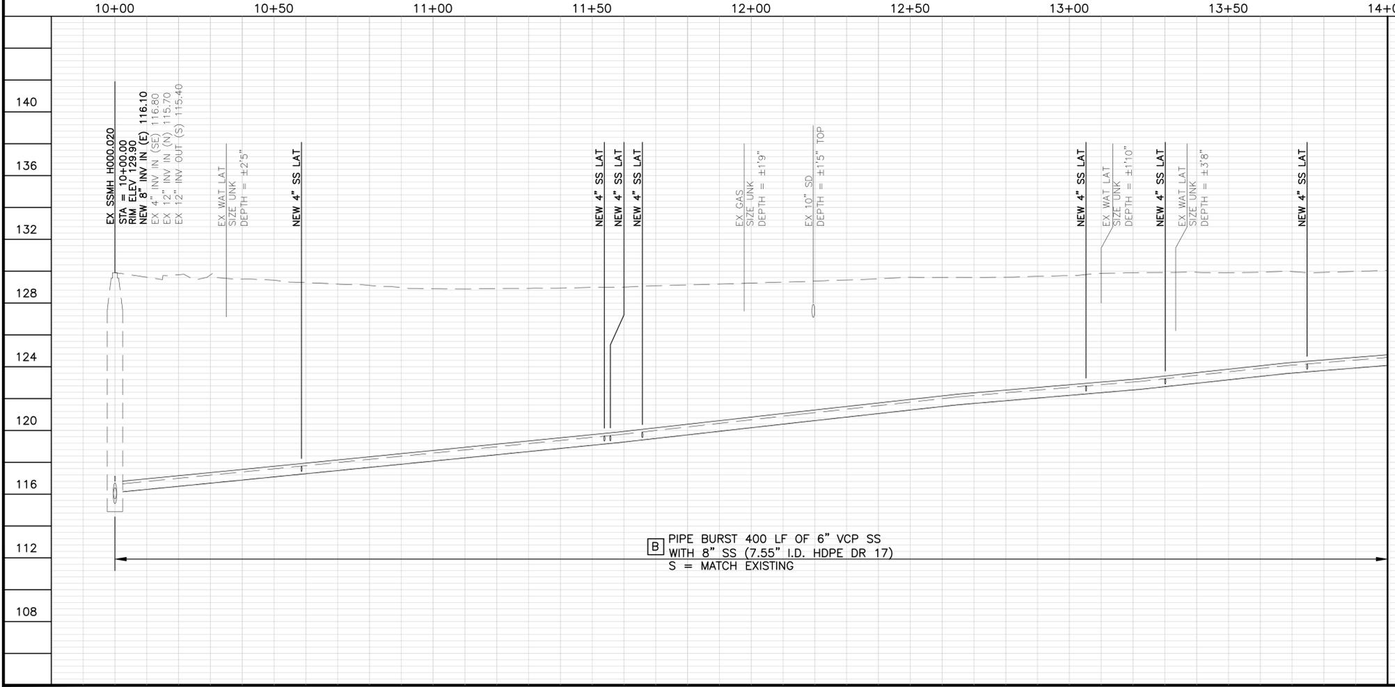
**B** PIPE BURST 400 LF OF 6" VCP SS WITH 8" SS (7.55" I.D. HDPE DR 17) S = MATCH EXISTING
