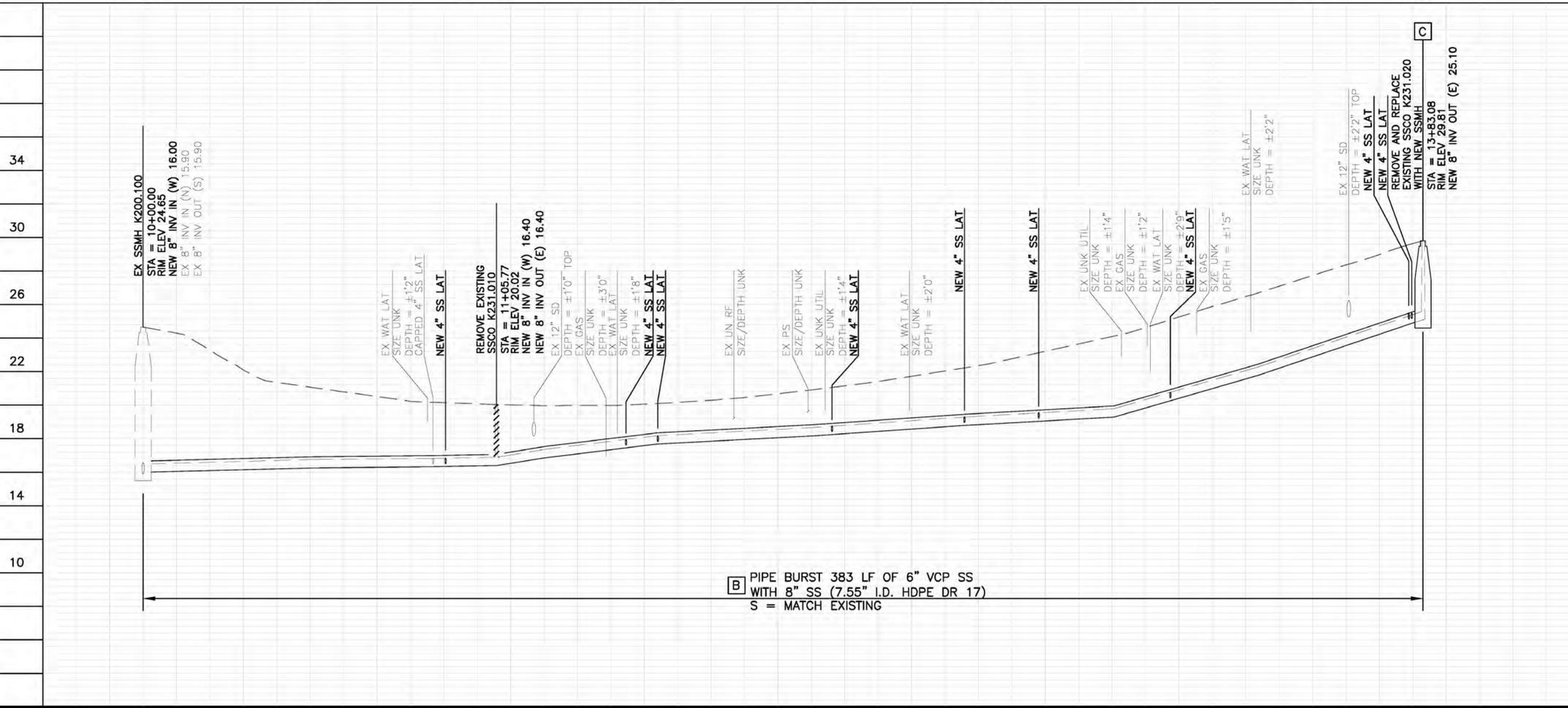
**B** PIPE BURST 383 LF OF 6" VCP SS WITH 8" SS (7.55" I.D. HDPE DR 17) S = MATCH EXISTING
