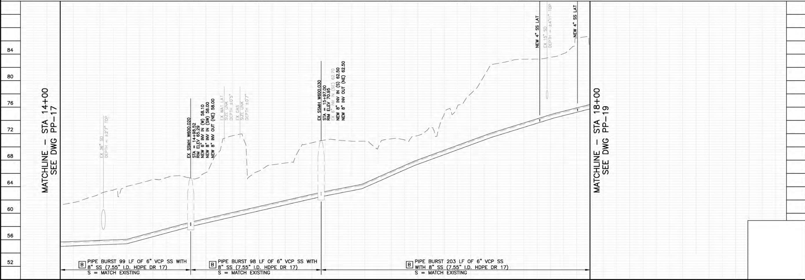
**B** PIPE BURST 99 LF OF 6" VCP SS WITH 8" SS (7.55" I.D. HDPE DR 17) S = MATCH EXISTING
