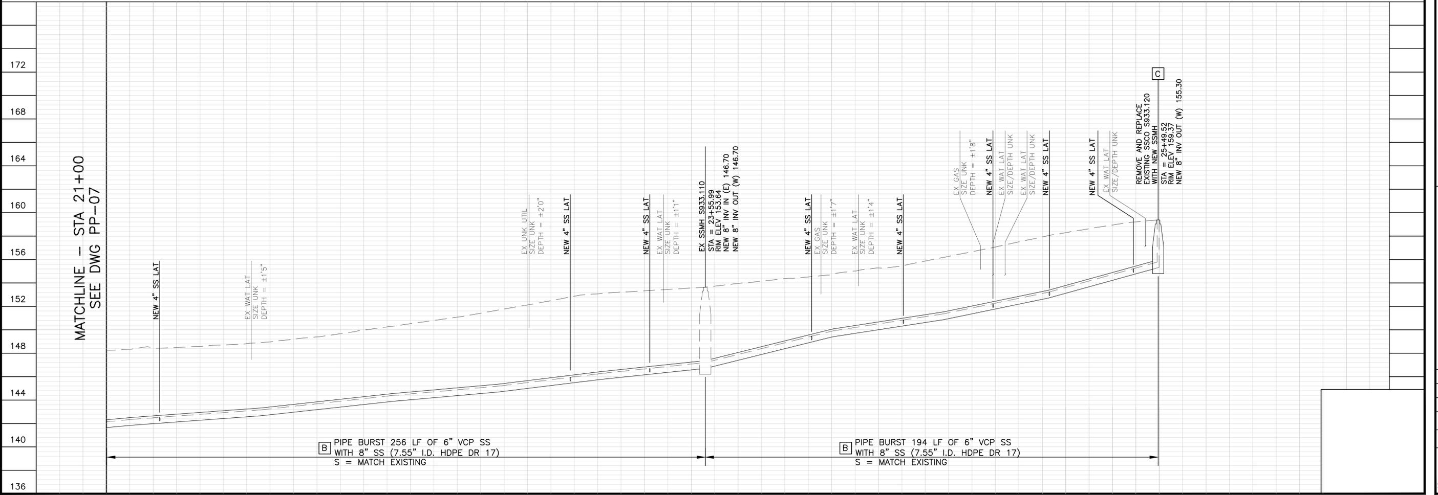
**B** PIPE BURST 256 LF OF 6" VCP SS WITH 8" SS (7.55" I.D. HDPE DR 17) S = MATCH EXISTING
