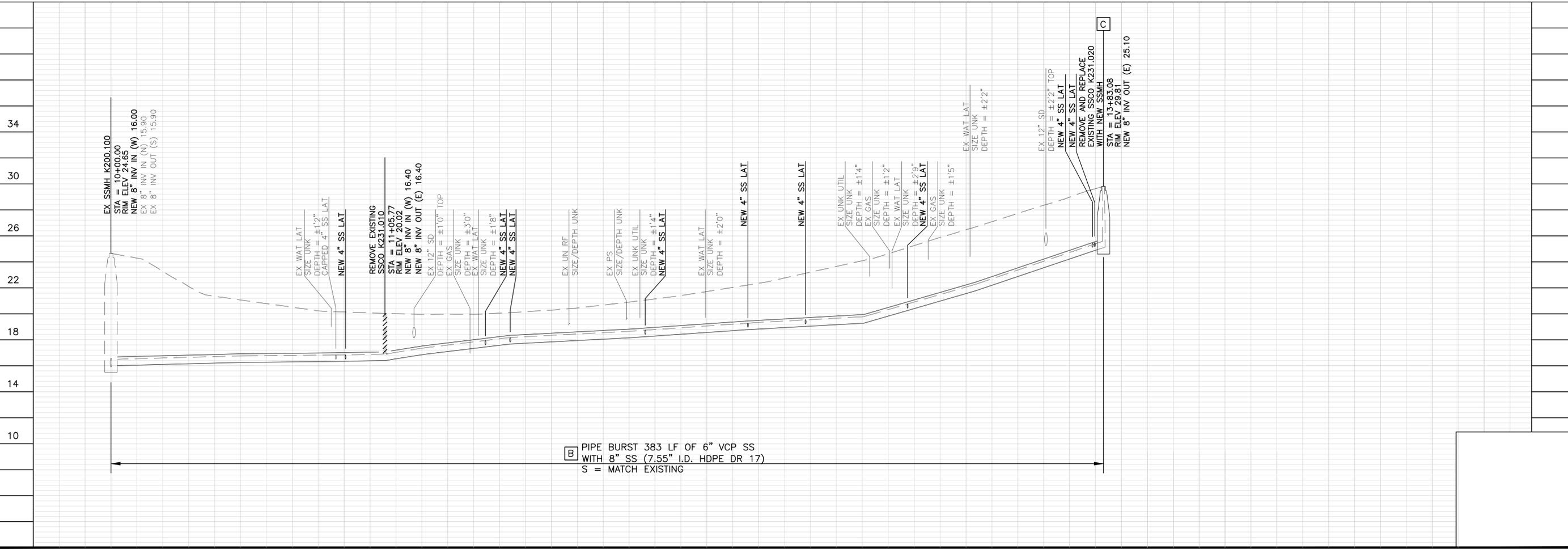
**B** PIPE BURST 383 LF OF 6" VCP SS WITH 8" SS (7.55" I.D. HDPE DR 17) S = MATCH EXISTING
