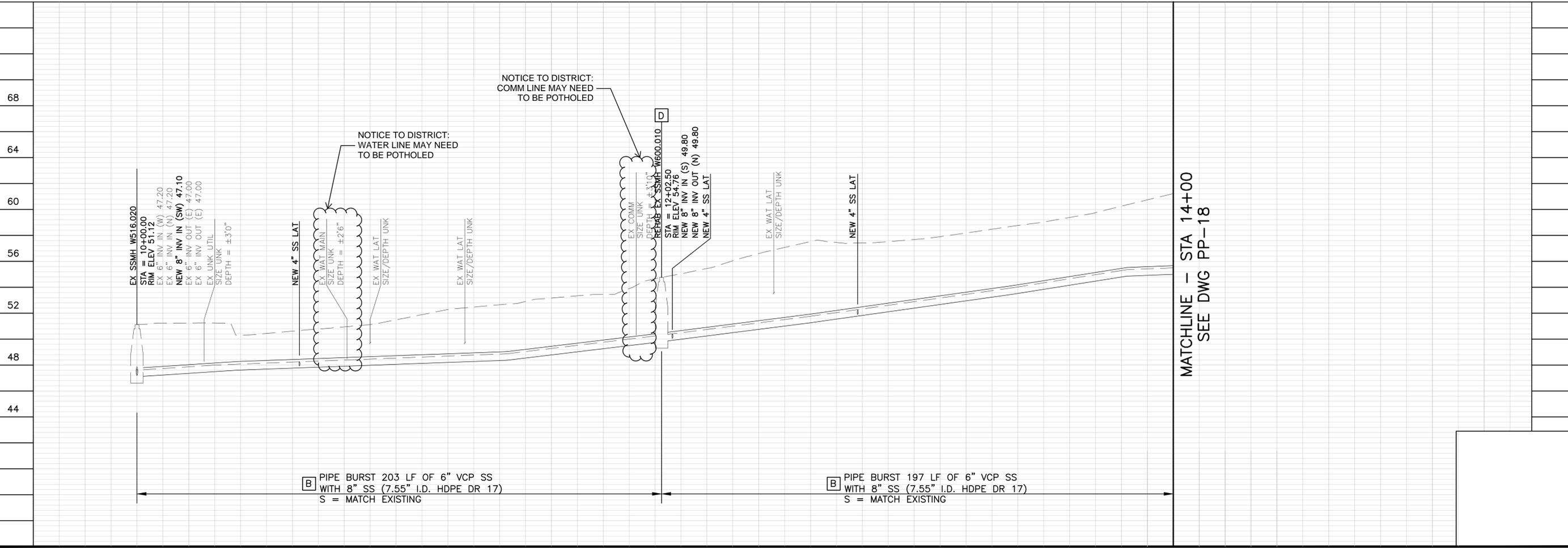
**B** PIPE BURST 203 LF OF 6" VCP SS WITH 8" SS (7.55" I.D. HDPE DR 17) S = MATCH EXISTING
