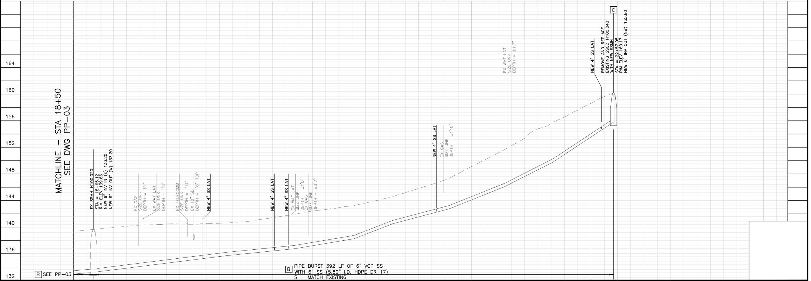
**B** PIPE BURST 392 LF OF 6" VCP SS WITH 6" SS (5.80" I.D. HDPE DR 17) S = MATCH EXISTING
