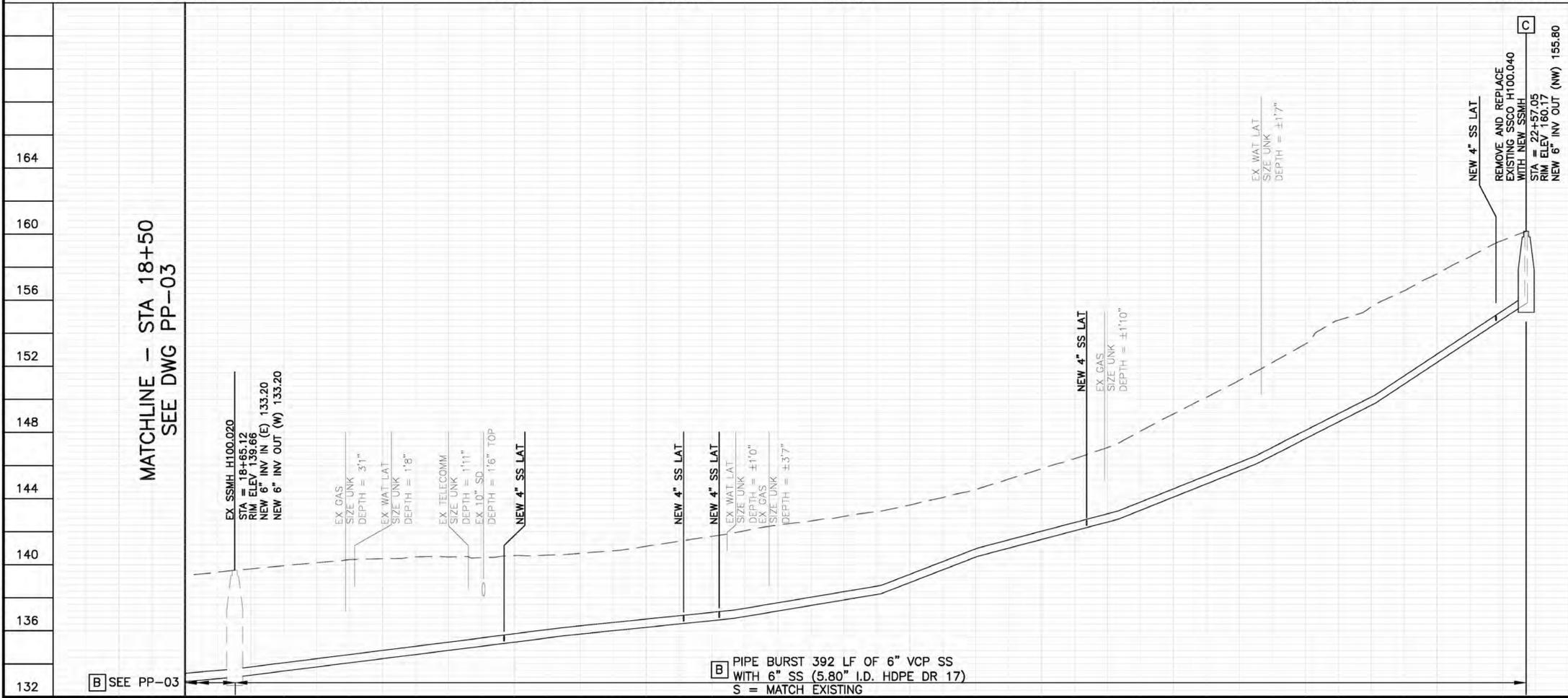
**B** PIPE BURST 392 LF OF 6" VCP SS WITH 6" SS (5.80" I.D. HDPE DR 17) S = MATCH EXISTING
