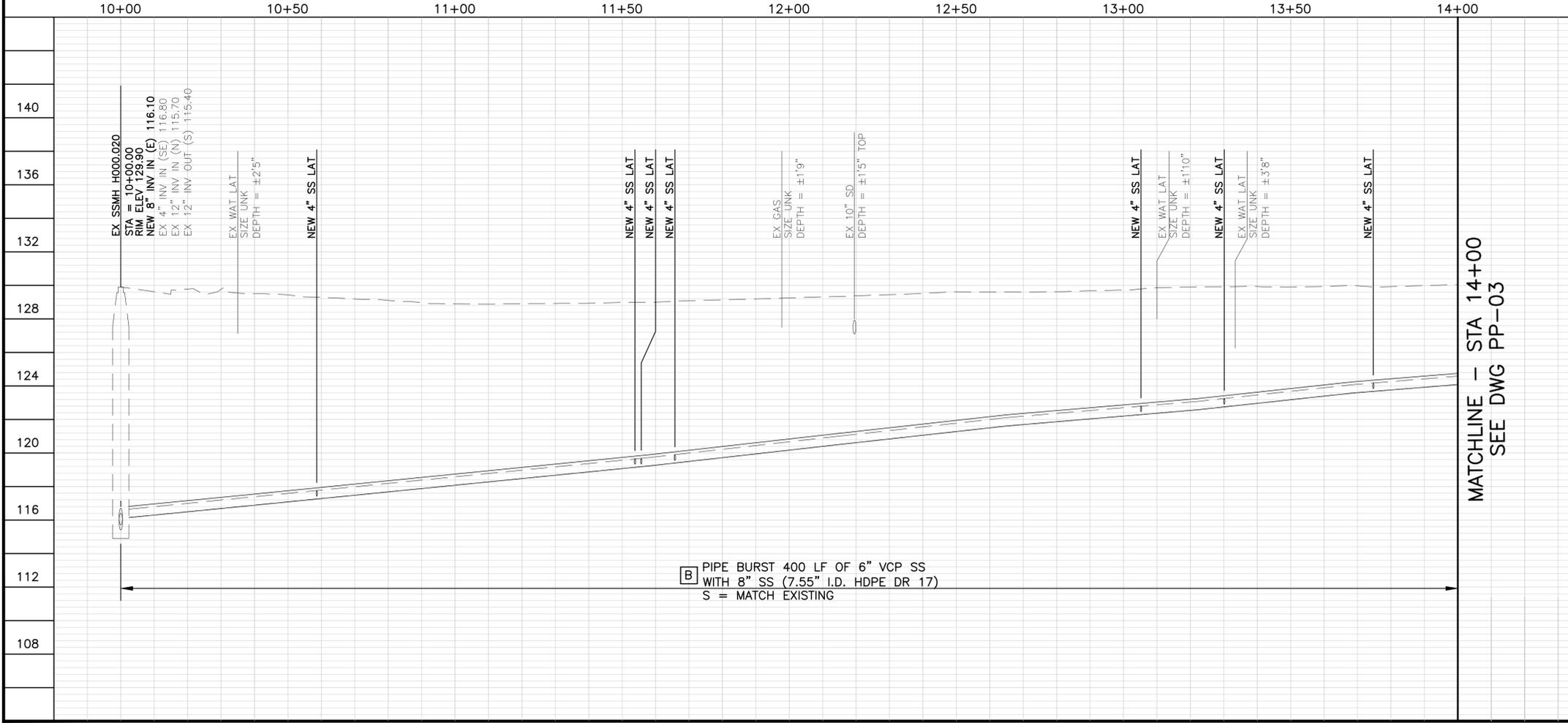
**B** PIPE BURST 400 LF OF 6" VCP SS WITH 8" SS (7.55" I.D. HDPE DR 17) S = MATCH EXISTING
