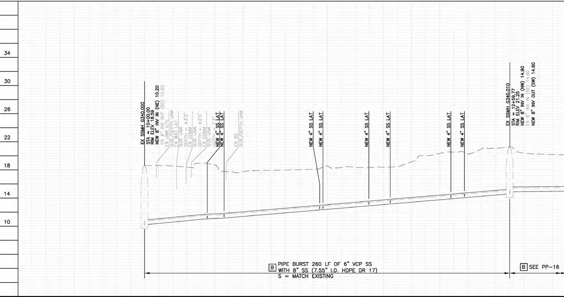
**B** PIPE BURST 260 LF OF 6" VCP SS WITH 8" SS (7.55" I.D. HDPE DR 17) S = MATCH EXISTING
