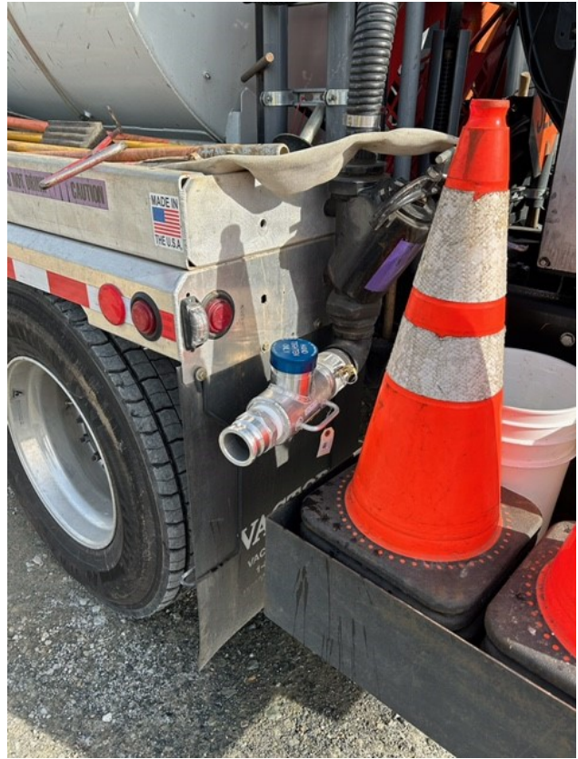
De-chlorination diffuser installed on the Ramjet Jetter.
